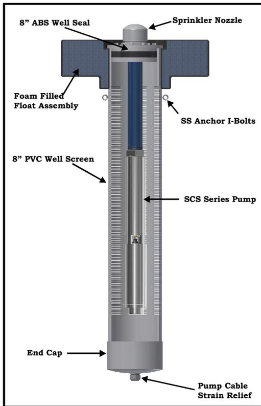
**SunPumps** SPF series solar powered pond fountains and aerators are the ultimate in performance and reliability. There are a variety of choices from ½ to 3 HP pumps, flow rates from 20 GPM to 130 GPM and choice of five different spray patterns.
